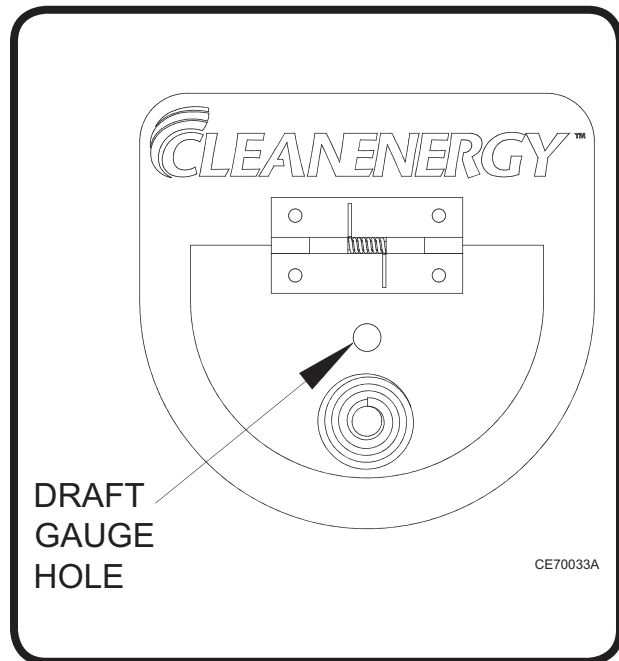
Figure 27: Draft Gauge Hole in the Observation Port
